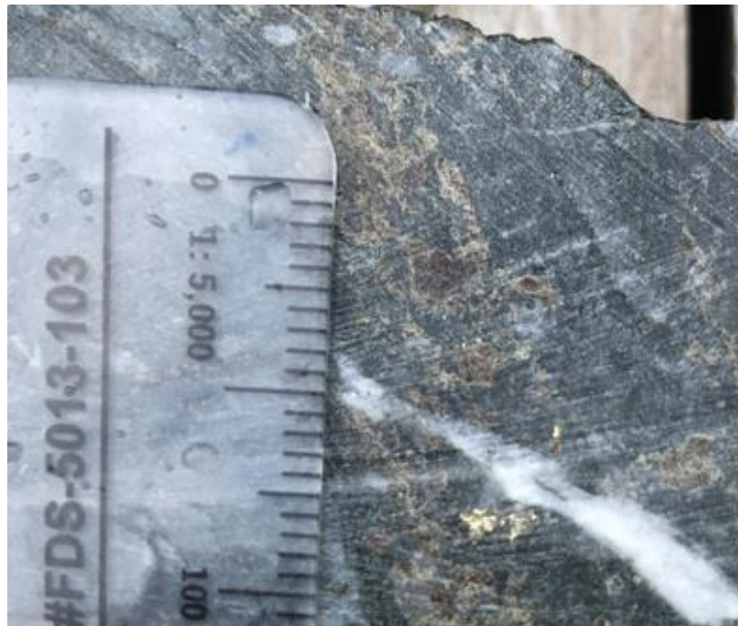
Figure 3 Image of visible gold grain in drill core from drill hole P20-2213 at a depth of 161.97m down the hole. The gold particle is associated with sphalerite, a zinc sulfide mineral, and quartz stockwork.
